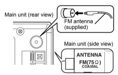
Stretch out the FM antenna to the best position for radio reception, and then fix it with adhesive tape.
